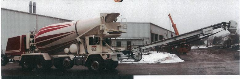
Front Discharge Conveyor uses innovative technology to make short work of long reaches.
